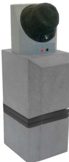
The unique properties of this low-mid frequency source include human body diffraction simulation, time stable sensor sensitivity and high noise levels. These features make this device extremely accurate and efficient for the analysis of transport vehicles like cars, vans, trucks, busses, trains and aircraft.
