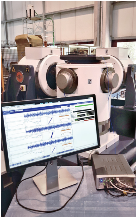
Using Simcenter SCADAS and Simcenter Testlab for MIMO 3D shaker control.
