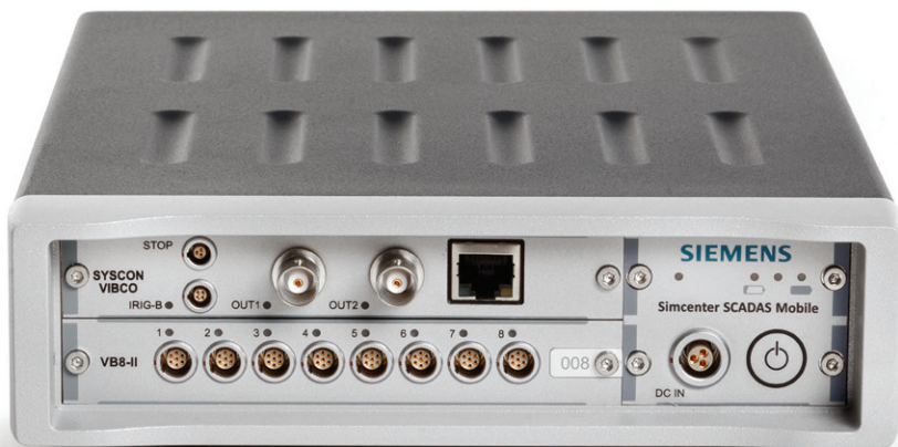
Simcenter SCADAS SCM201V with eight-channel acquisition module.
