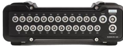
Units connect in daisy chain to a Recorder unit for autonomous operation or in combination with a PC, tablet, or smartphone.
